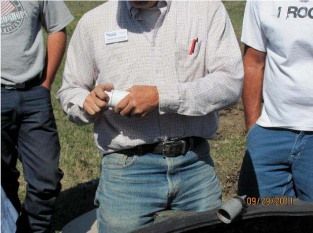
Herschel is holding the break away section he recommends to protect the valve and pipe threads.
