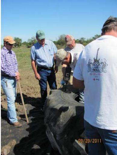
It helps to have at least one other person to stabilize the saw and lubricate the blade as the cut is being completed. Supporting the cut part of the tire will also help prevent binding on the blade.
