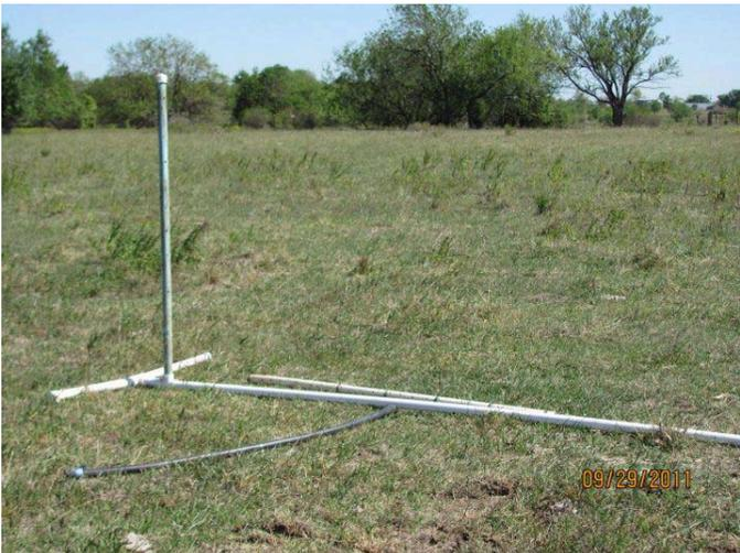
If the pond is not fenced, this assembly should be protected and supported by posts or other supports.
