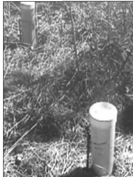
*Groundwater samplers were placed at one foot and two foot depths on the Kunard site.*
