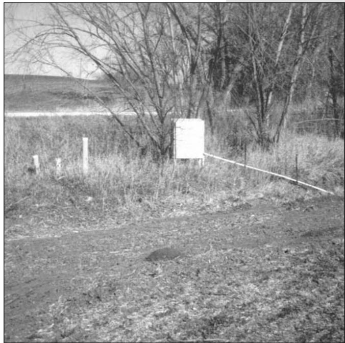
*Runoff and groundwater samplers were placed at the bottom of a waterway on the Peters' site to assess water quality flowing through the waterway, and groundwater moving to the nearby stream.*
